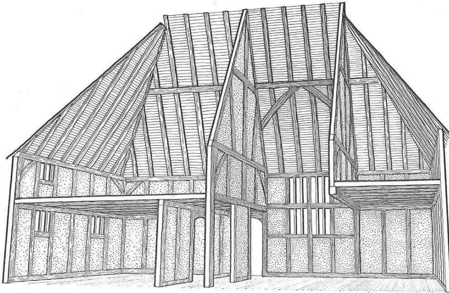
A cutaway drawing showing the probable extent of a late phase in the development of the medieval timber-framed building.
